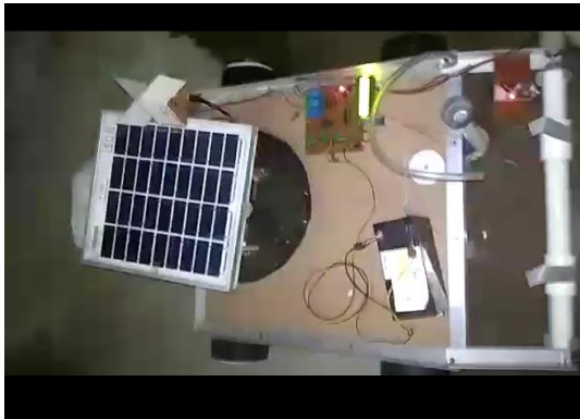
Figure 3. Smart agricultural mobile operated robot powered by solar energy
